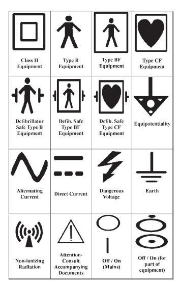
Fig. | British Standard Symbols used on medical equipment.
